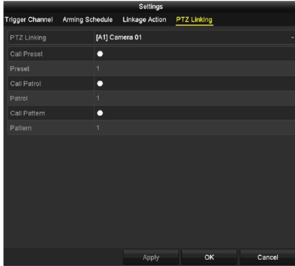
Figure 8-9 Set PTZ Linking of Alarm Input
