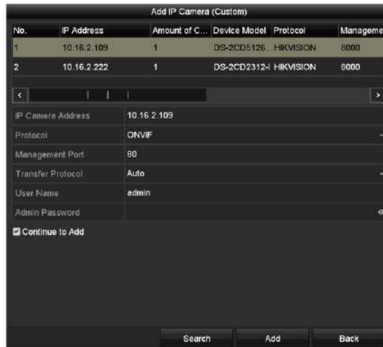
Figure 2-38 Custom Adding IP Camera Interface
