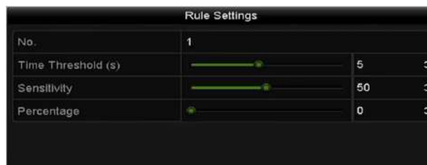
Figure 9-8 Set Intrusion Crossing Detection Rules
