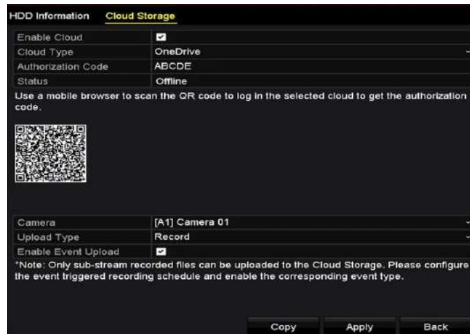
Figure 12-20 Upload to Cloud Storage Interface
