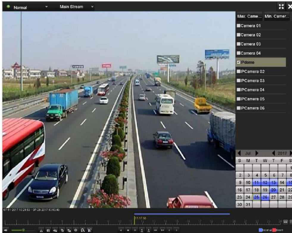
Figure 6-9 Interface of Playback by Time
