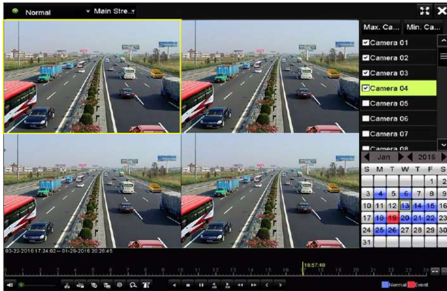
Figure 6-24 4-ch Synchronous Playback Interface
