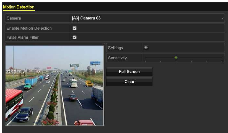
Figure 8-1 Motion Detection Setup Interface
