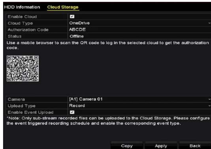
Figure 12-18 Cloud Storage Interface
