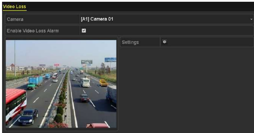
Figure 8-12 Video Loss Setup Interface
