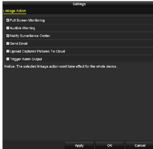
Figure 8-11 Disarm Linkage Actions
