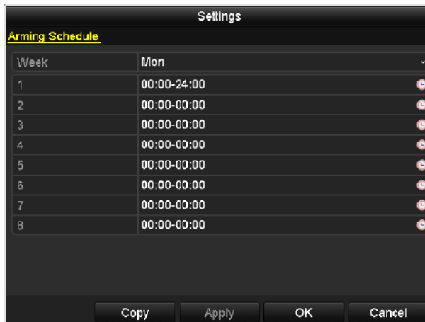
Figure 8-22 Set Arming Schedule of Alarm Output
