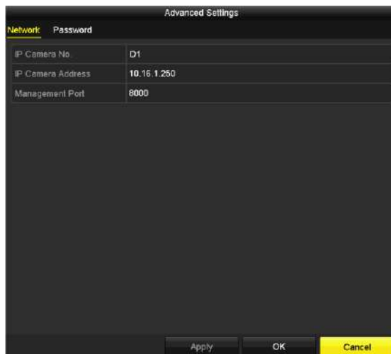
Figure 2-41 Network Configuration of the Camera
