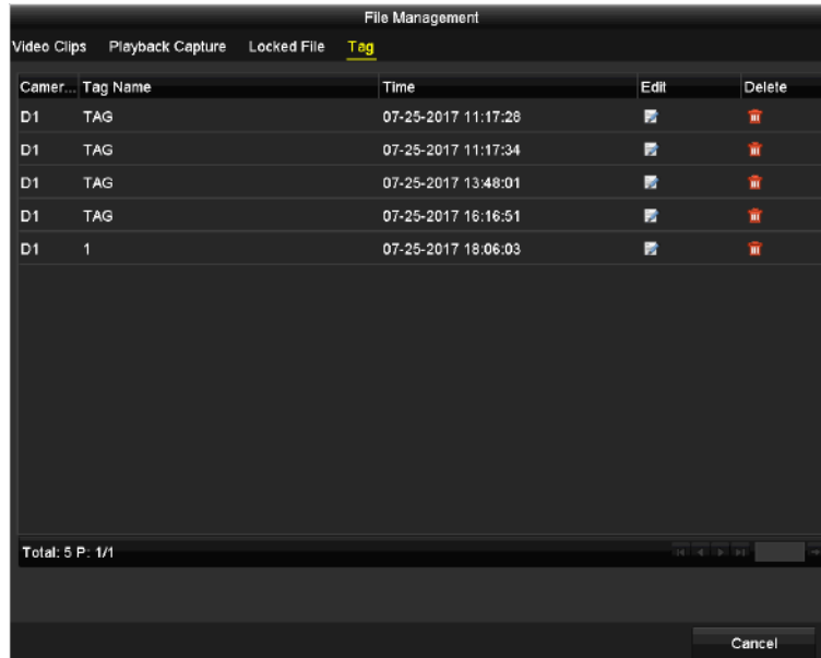
Figure 6-11 Tag Management Interface
