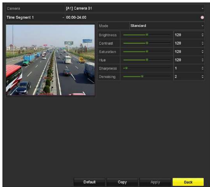
Figure 13-5 Image Settings Interface (Analog Camera)
