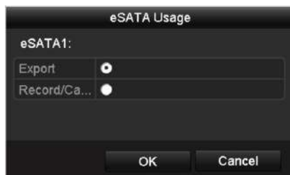
Figure 12-23 Setting eSATA Usage
