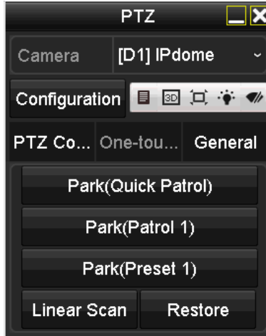
Figure 4-12 PTZ Panel - One-touch
