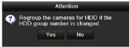
Figure 12-14 Confirm HDD Group Settings
