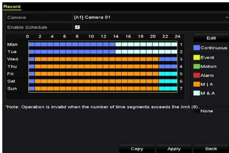
Figure 5-12 Draw the Recording Schedule
