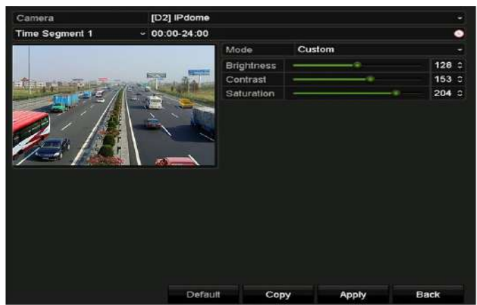
Figure 13-6 Image Settings Interface (IP Camera)
