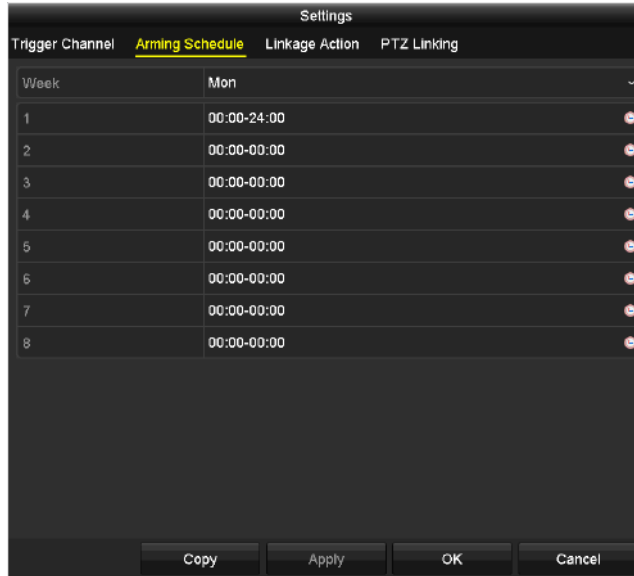
Figure 8-8 Set Arming Schedule of Alarm Input
