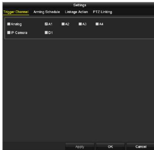
Figure 5-21 Set Triggered Camera of VCA Alarm
