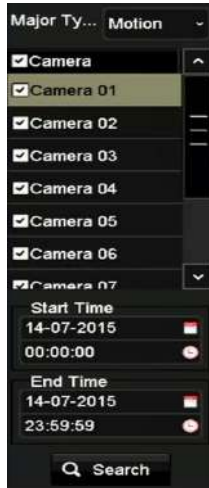
Figure 6-6 Video Search by Motion Detection
