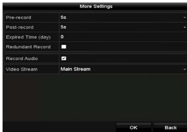
Figure 5-5 More Settings of Record Parameters
