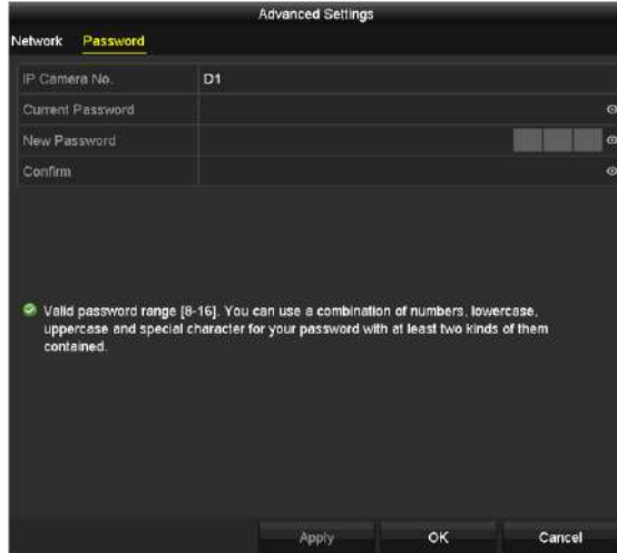
Figure 2-42 Password Configuration of the Camera
