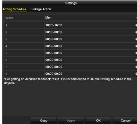
Figure 8-17 Set Arming Schedule of Video Quality Diagnostics
